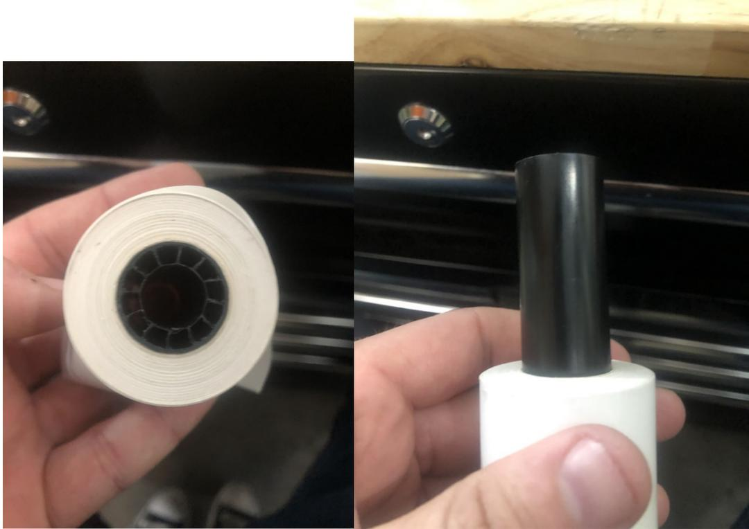
Once it is out you will need to put the plastic piece from the inside of the machine in the center of the roll. Place the 2 sides of the plastic in the channels by the receipt paper.
