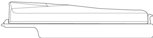
Press tab to remove scanner from Klip Case.
