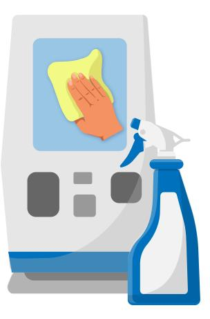
Spray cleaning solution\* onto cloth and wipe screen. Do not spray cleaning solution directly onto the touch screen.
