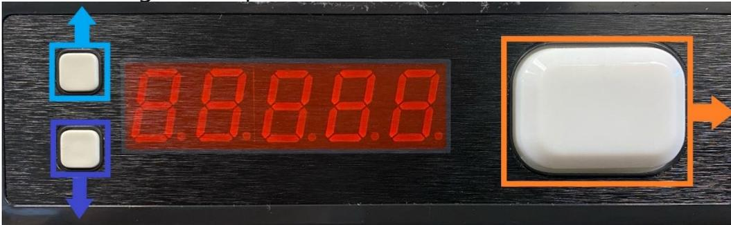
5. After setting the desired number, tap the big button until the Light turns off to finalize the programming.
