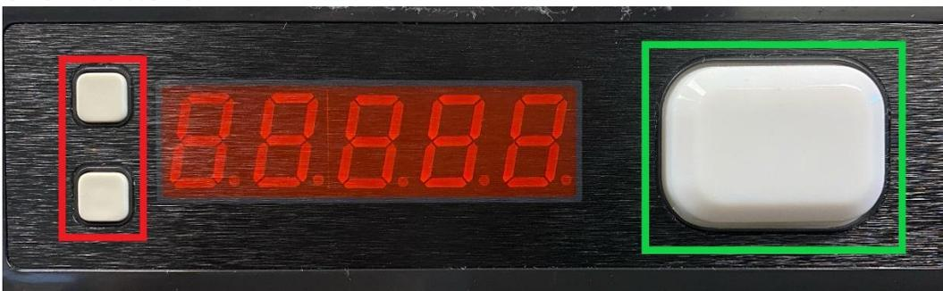
3. If done correctly the light will be in programming mode and display its current number.
