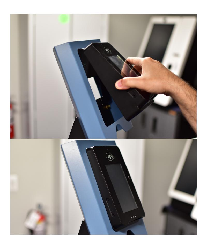
**Step 4**Install the four M3 screws to secure the PicoMarket to the stand.
