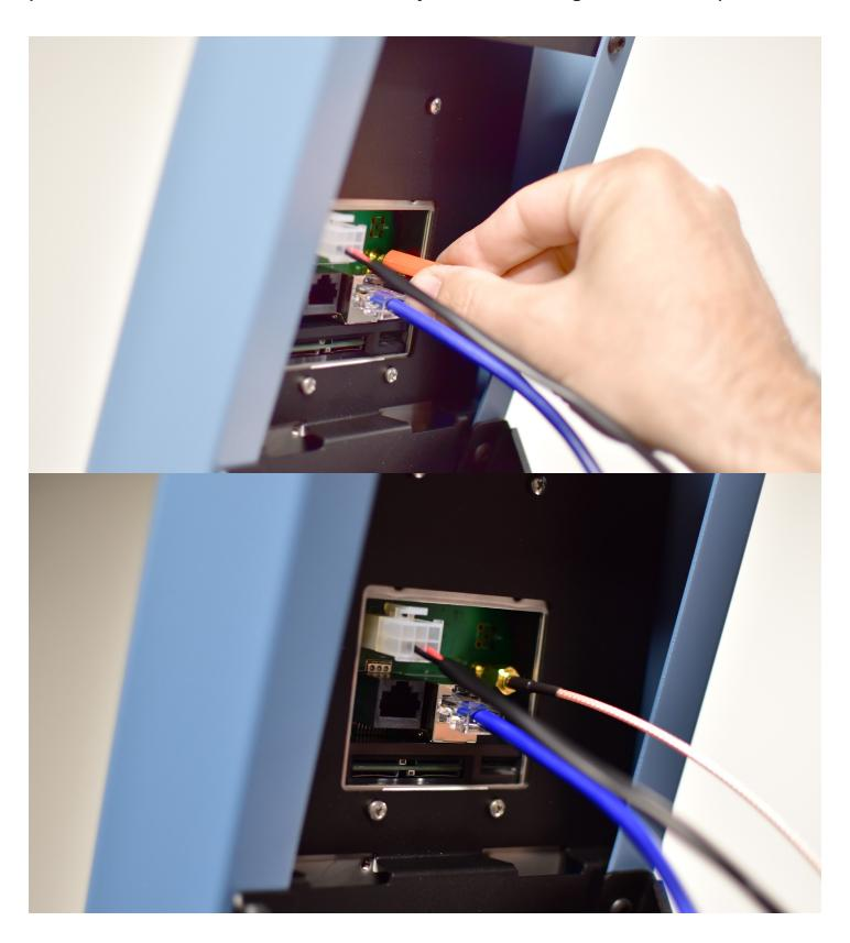
**Step 8**Fit the wire loom over the cables.
