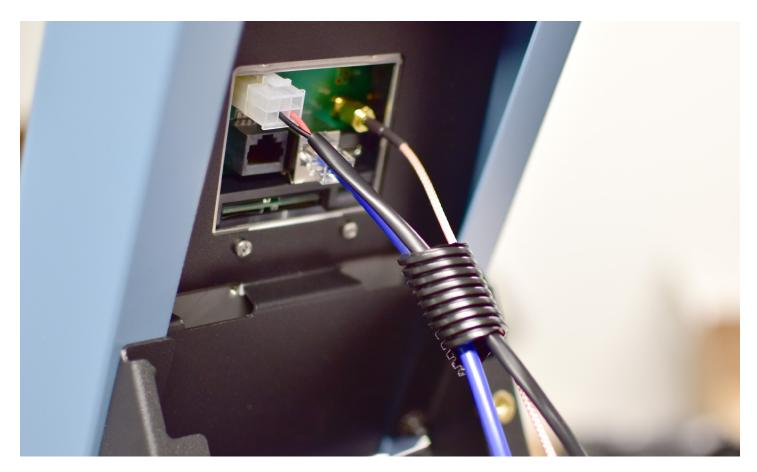
**Step 9**Reinstall the PicoMarket backplate and insert the philips screw.
