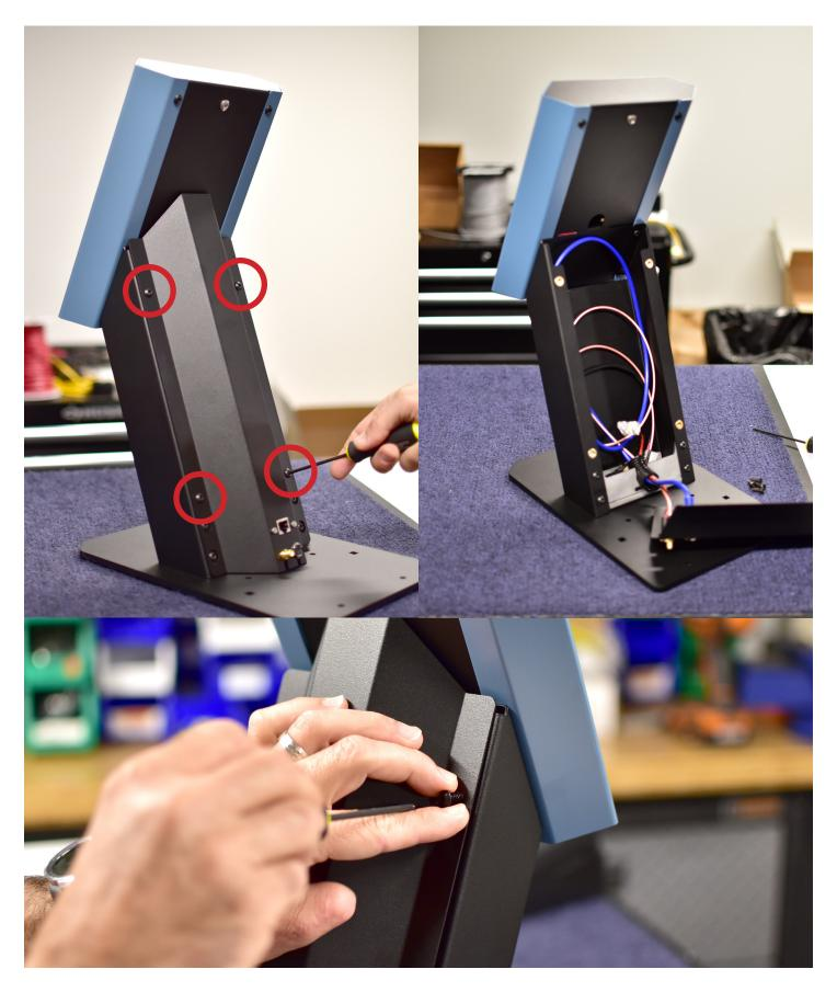
**Step 2**Remove the cover from the PicoMarket housing by removing the philips screw.
