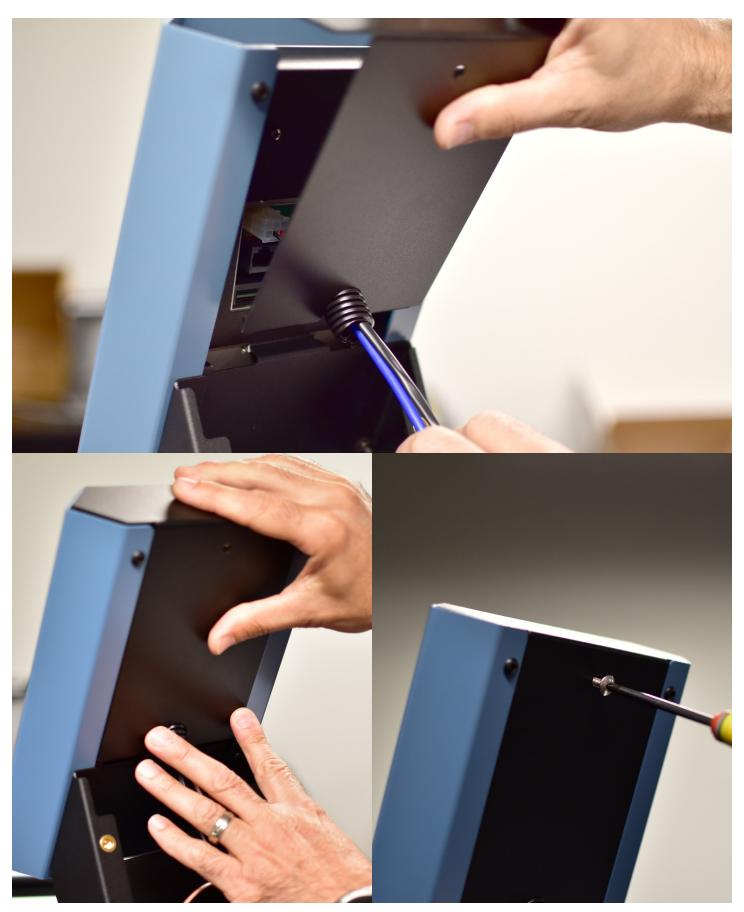
**Step 10**Ensure all cables are tucked inside the PicoMarket stand and reinstall stand backplate and screws.
