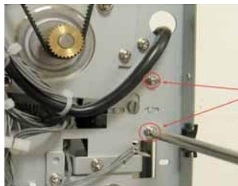
5. Turn the adjustment cam (shown) very slightly, to cause a change in the value of the sensor output.
