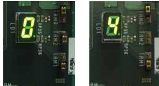
10. The easiest way to remove the thickness gauge, pull the jumper back off when the display reaches zero. This will run the continuous motor test and will send the note to the reject bin.
