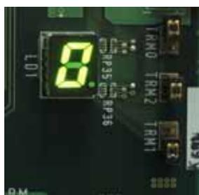
3. RAS mode 9 will display the current value of the thickness sensor level. Since there is only one digit, it will alternate between the two values as shown in the pictures. This is a hex value and SHOULD be in the range of E5 to E9
