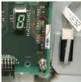
2. Now turn the power ON, and watch the LED cycle from 0 through B and then start over.
