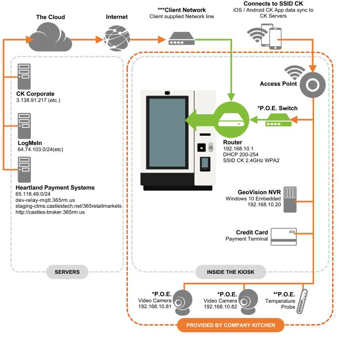
\* Power Over Ethernet (POE) connections to power the cameras
